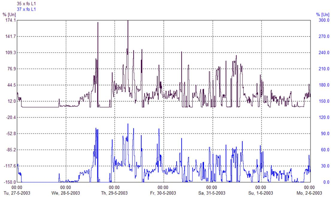
**Figure 3 – 35<sup>th</sup> and 37<sup>th</sup> voltage harmonics measured in Wind Turbine 2**
