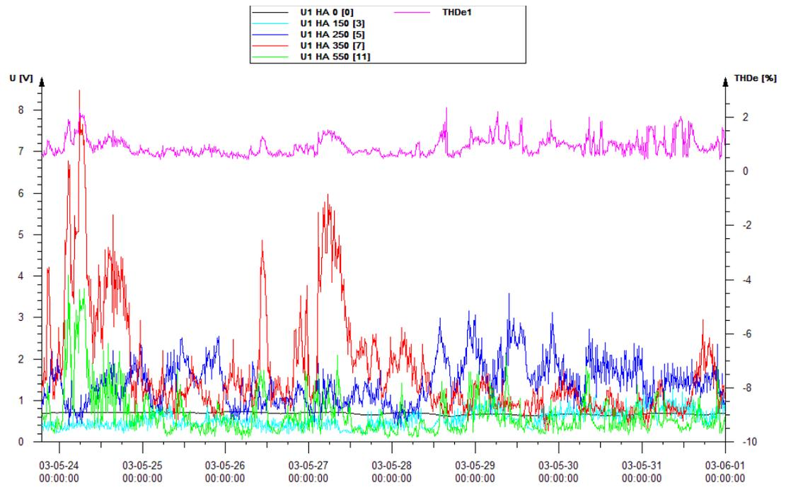
**Figure 2 - European THD, 3<sup>rd</sup>, 5<sup>th</sup>, 7<sup>th</sup> and 11<sup>th</sup> voltage harmonics, and DC component measured in the output of Wind Turbine 1.**
